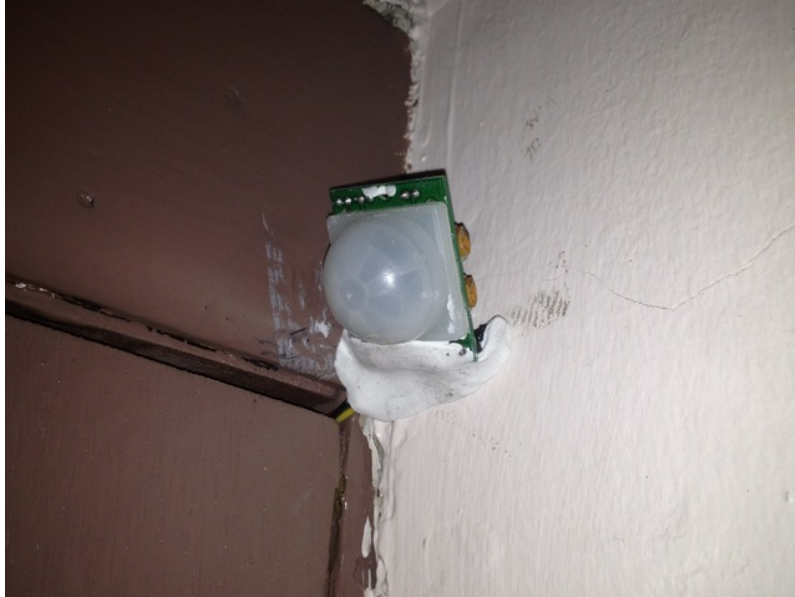
Mounted PIR sensor with some Sugru (http://adafru.it/436)
