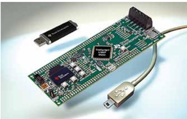
The EK-LM4F232 Development Kit is a compact and versatile tool for the Tiva C Series TM4C123G ARM® Cortex™-M4F based MCU. Key highlights include a color OLED display, USB OTG, a micro SD card, a coin cell battery for use with low-power hibernate, a temperature sensor, a three axis accelerometer for motion detection, and easy-access through-holes to all of the available device signals.
