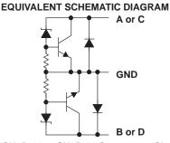
(One SN65240 or SN75240 Suppressor Shown) NOTE: All four GND terminals should be connected to ground.
