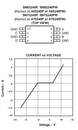
NOTE A: Typical current versus voltage curve was derived using the IEC 1.2/50-µs surge waveform.
