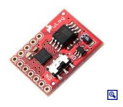
The uLog is a tiny analog-voltage logger with a 3.3V TTL serial interface. It uses an Atmel ATtiny24 AVR to sample three analog voltage channels at 50 Hz with 10-bit resolution and stores the data on an AT45DB161D 16 Mbit flash IC, which allows for approximately two hours of logging when running the default firmware.
