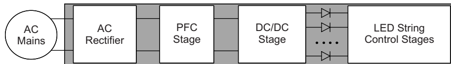
Figure 2. Block Diagram for a Typical LED Lighting Application
