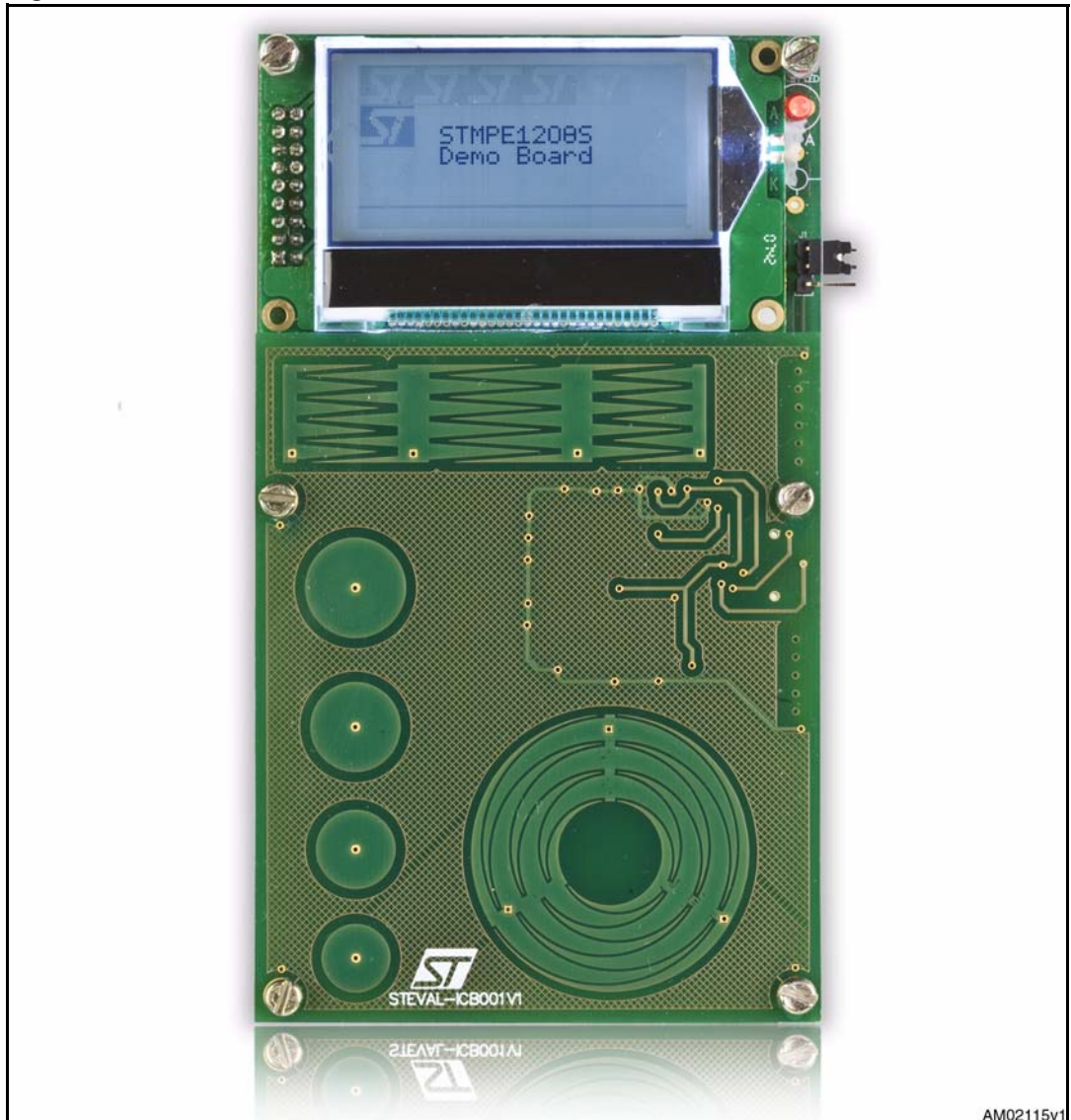
Figure 1. STEVAL-ICB001V1 touch sensor demonstration board
