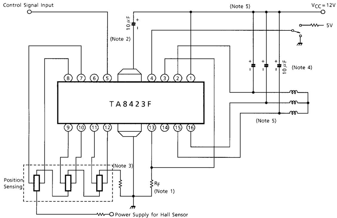
Note 1: Recommendable value of  $R_F$  is 0.3 to 5  $\Omega$ . It depends on required initial torque, gain, coil impedance and control voltage of Pin 5.
