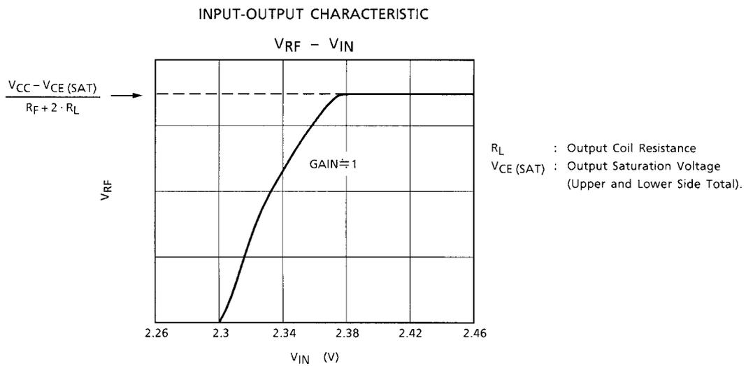
$V_{RF}$  is feed back voltage generated by  $R_F$  and output current of  $I_L$ , drive current of  $I_D$  and internal reference circuit current of  $I_R$ .
