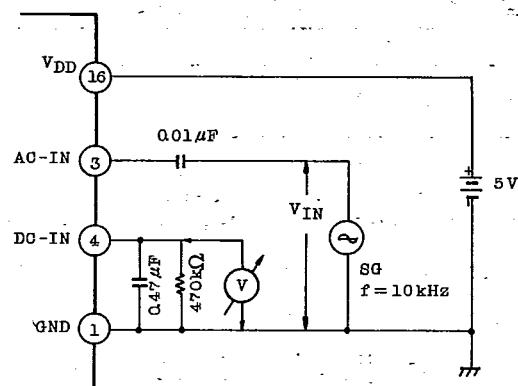
\* An output value of SG when 4.5V is generated at DC-IN is denoted by VIN.
