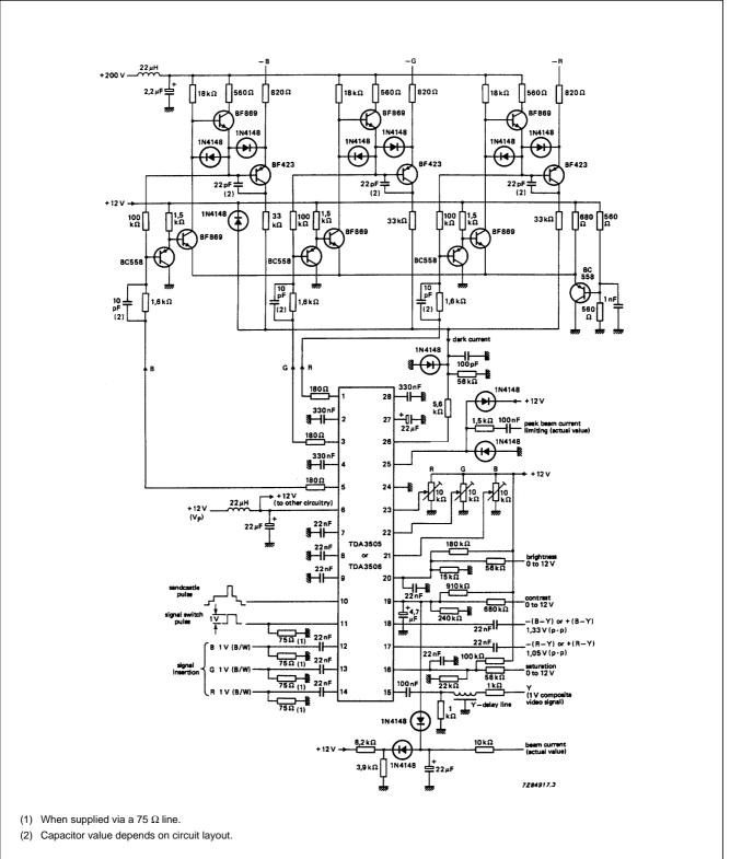
Fig.3 Typical application circuit diagram using TDA3505 or TDA3506; colour difference inputs are negative for TDA3505 or positive for TDA3506.
