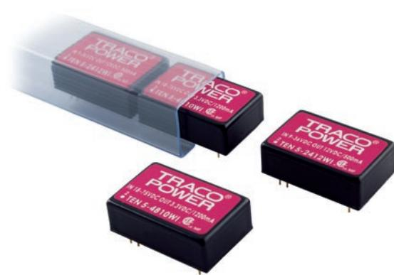
The TEN 5WI series is a family of high performance dc-dc converter modules with 5 W output power, featuring ultra wide input voltage ranges of 9 - 36 VDC or 18 - 75 VDC. They come in a shielded DIP-24 metal package with industry-standard footprint.
