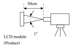
Luminance Meter (TOPCON BM-5A) Spectroradiometer(TOPCON SR-3)
