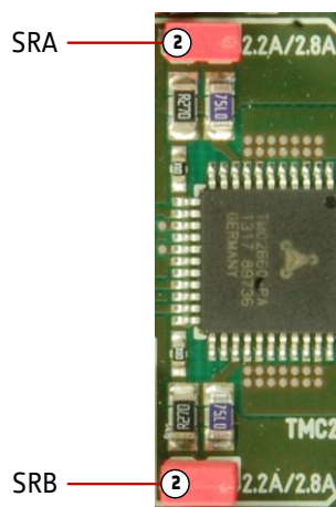
Figure 3.11 Chopper test points
