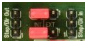
Figure 3.7 Jumper setting for TMC4210 selection.
