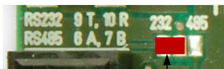
Solder bridge for RS232
