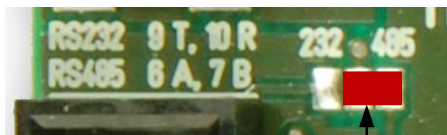
Solder bridge for RS485
