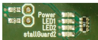
Figure 3.10 LEDs of TMC4210+TMC2660-EVAL
