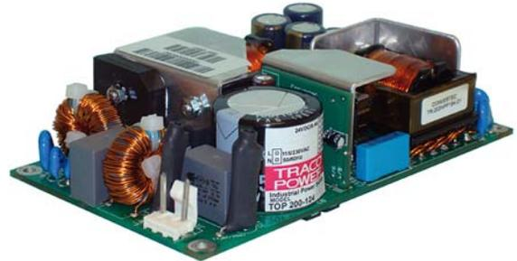
The new TOP-200 Series AC/DC Power Supplies feature the highest power rating in the industry standard 3.0" x 5.0" (76.2 x 127 mm) footprint. They can supply up to 200 W output power with convection cooling over an industrial operating temperature range of -25°C to +70°C. This performance could be realized by a state of the art design providing an extremely high efficiency of >90 % which eliminates the need for a dedicated power supply cooling fan.
