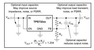
Figure 32. Typical Application Circuit for Adjustable-Voltage Versions
