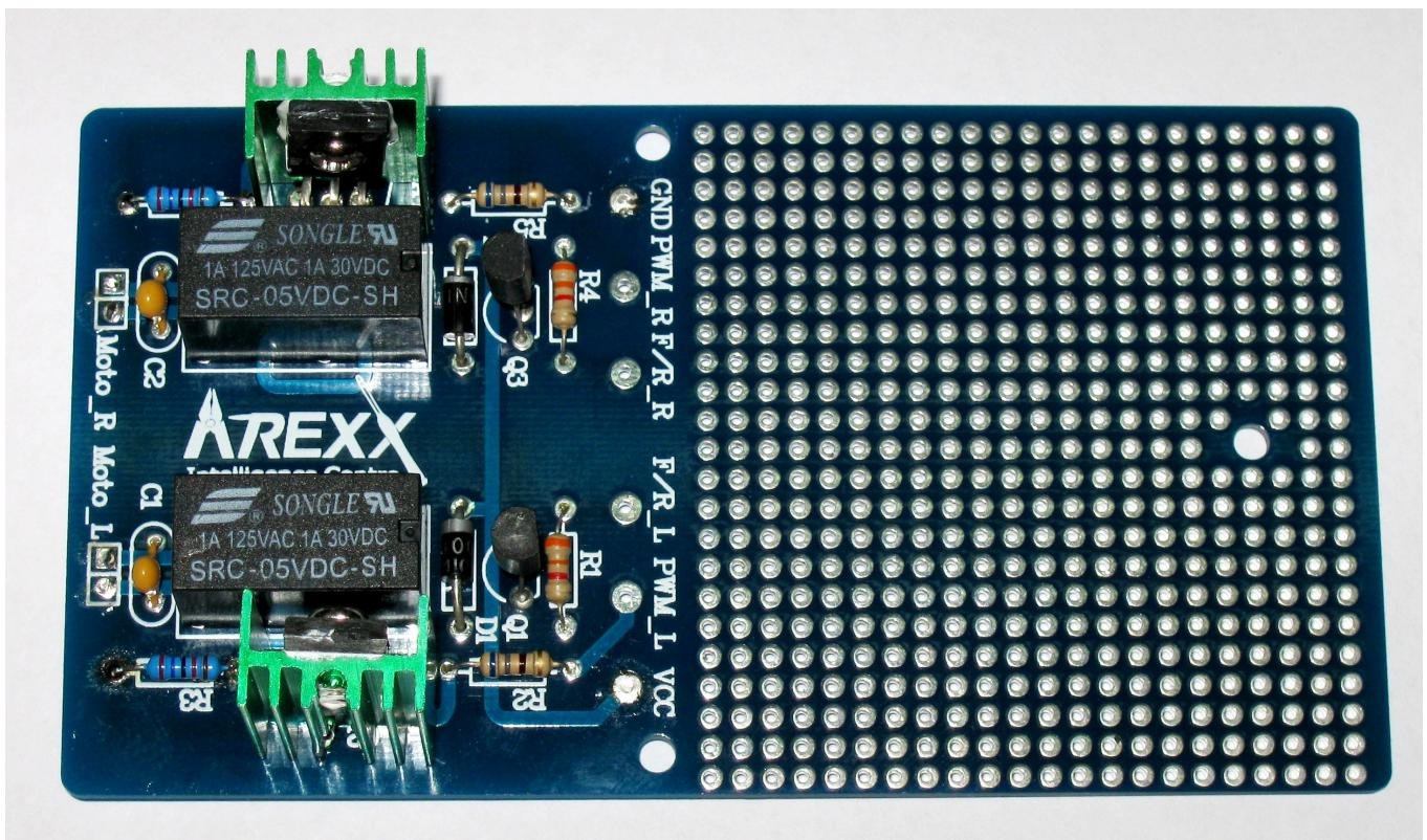
This is the **Dagu Mr. Basic Dual 2A Motor Controller Board**. This simple motor controller PCB is designed specifically for Mr. Basic. Capable of working from 3.6V - 6V this PCB provides speed (PWM) and direction control of 2 motors with up to 2A per motor. Over half of the PCB is double sided project board with plate through holes for maximum versatility. This board requires soldering. It is supplied in re-sealable plastic bag with cardboard header.
