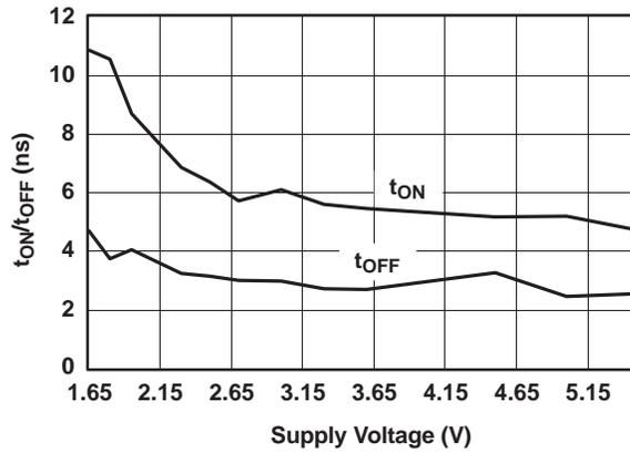
Figure 6. t<sub>ON</sub> and t<sub>OFF</sub> vs V<sub>+</sub>
