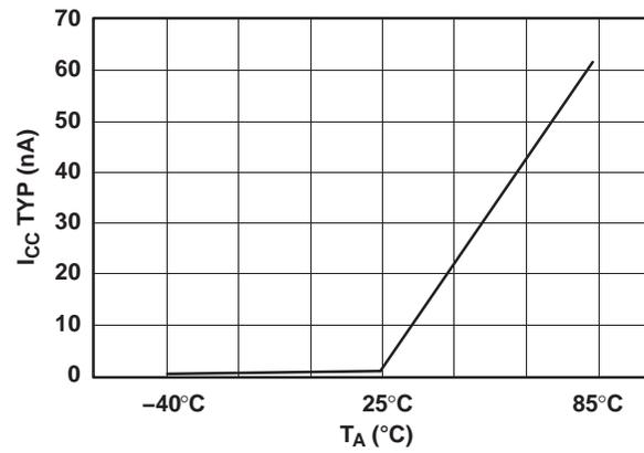
Figure 12. Power-Supply Current vs Temperature
