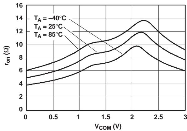
**Figure 2.  $r_{on}$  vs  $V_{COM}$  ( $V_+ = 3\text{ V}$ )**
