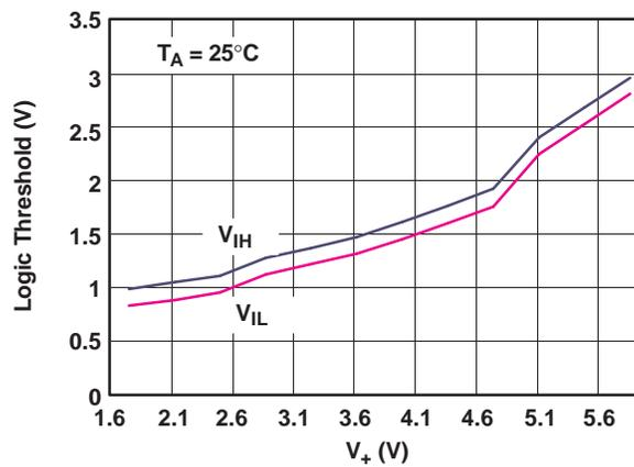
Figure 8. Logic Threshold vs V<sub>+</sub>
