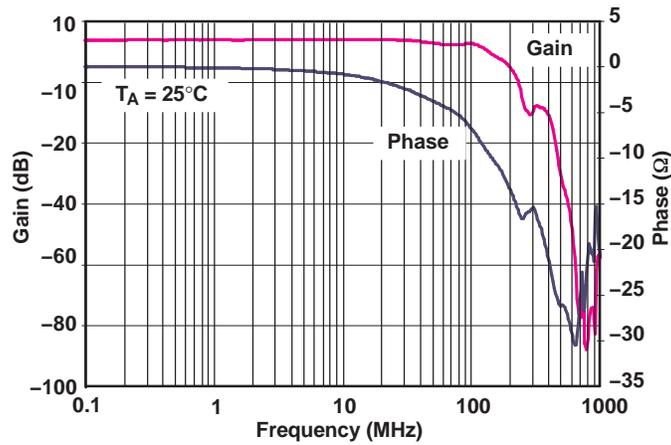
Figure 9. Bandwidth ( $V_+ = 5\text{ V}$ )
