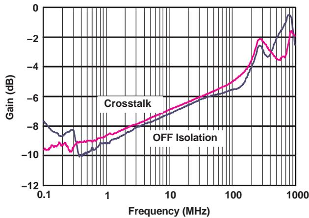
Figure 10. OFF Isolation and Crosstalk ( $V_+ = 5\text{ V}$ )
