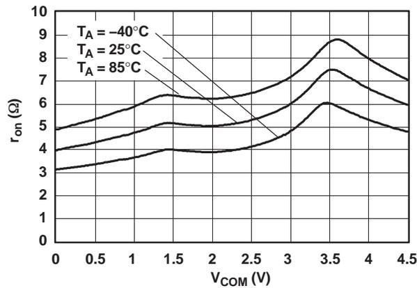
Figure 3.  $r_{on}$  vs  $V_{COM}$  ( $V_+ = 4.5$  V)
