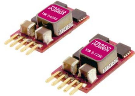
The new TSR-3 series dc/dc-converters are non-isolated step-down switching regulators for point of load applications. A high efficiency up to 95 % allows a full 3 A load operation up to +50°C ambient temperature without the need of any heat-sink or forced cooling.
