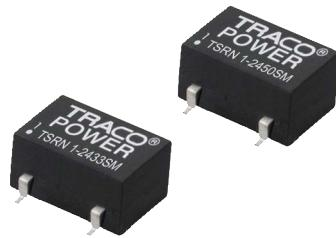
The new TSRN-1SM series are step-down non-isolated switching regulators in compact SMD package. They are an ideal solution to replace inefficient linear regulators. The high efficiency up to 95 % allows full load operation up to +55°C (+85°C with derating) ambient temperature without the need of forced aircooling.
