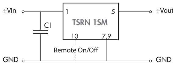
C1 = 22 µF / 50 V (required only if input voltage is higher than 36 V)
