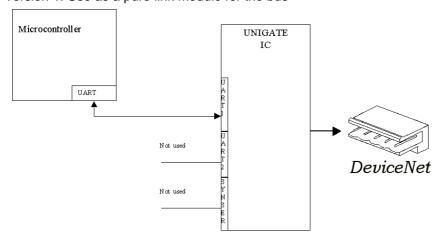
The UNIGATE® IC independently processes the communication with the customer's device via the TTL-interface.
