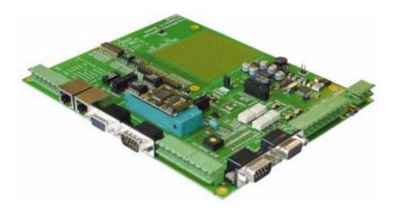
The required UNIGATE® IC / ICs are ordered separately. The required voltage (5V or 3.3V, depending on the version) can be adjusted. An RS232-interface or a USB-connection is available for the connection to the PC (Debug-interface).
