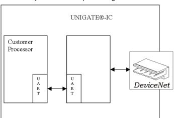
After the RS232-driver has been replaced by the UNIGATE® IC, the DeviceNet is available at the 5-pol. screw-plug connector.
