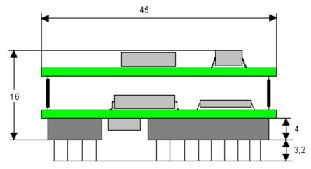
The pins of UNIGATE® IC - DeviceNet are arranged with a grid spacing of 2.54 mm.
