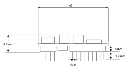
The pins of UNIGATE® IC are arranged with a grid spacing of 2.54 mm.
