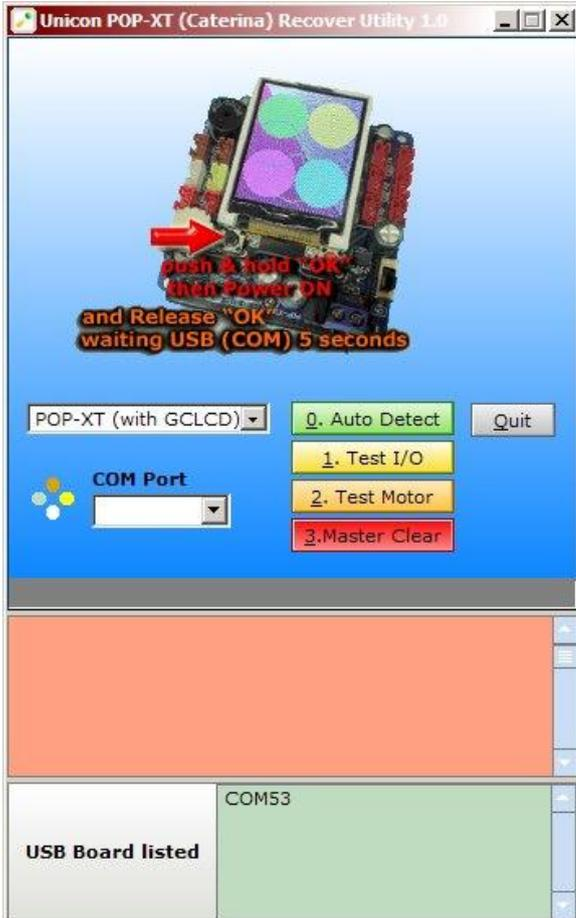
Two. Program will display COMPORT detected at the bottom of the screen as shown.
