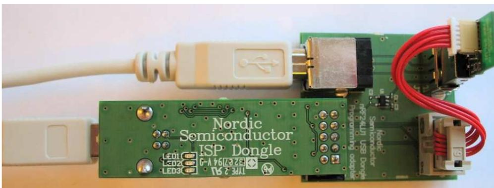
Figure 6 - nRF24LU1 USB Dongle Programming Adapter assembly
