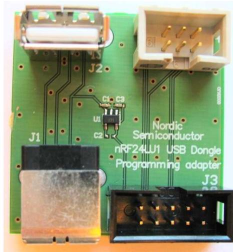
Figure 5 - nRF24LU1 USB Dongle programming adapter
