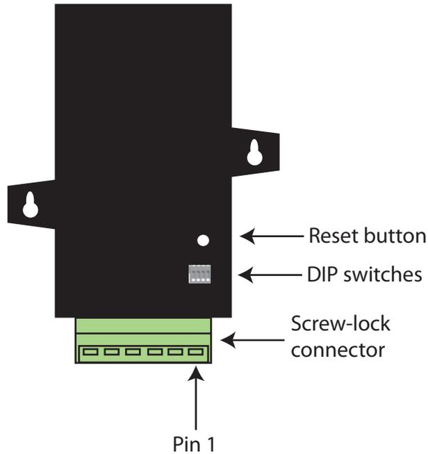
The adapter is switch-selectable between RS-422 half duplex/full duplex, and RS-485 modes (see "DIP switches" on page 25). The function for several pins varies between RS-422 and RS-485 modes.
