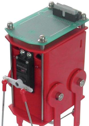
Installing experiment PCB
